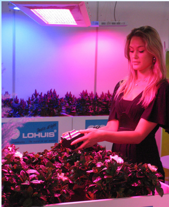
Figure 3. Measuring the output of LEDs used in greenhouse operations helps growers adjust LED output to optimize plant growth.
