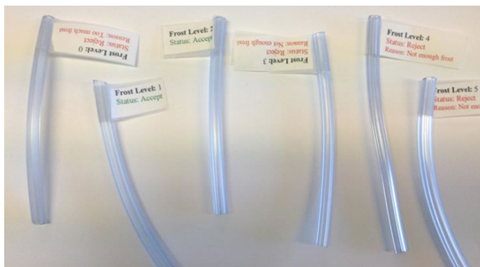
Figure 1: Although differences in the frosting levels of plastic tubing samples are difficult to distinguish visually, spectroscopic methods are highly reliable in characterizing tubing properties.
