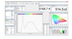
The S-BTS256 user software for the luminous flux with integrated and external sphere.
