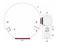
1) BTS256-LED 2) 50mm integrating spherel 3) Precision bayonet mount 4) BiTec sensor with Si photodiode, CMOS diode array spectrometer and shutter 5) Microprocessor 6) USB interface 7) ISD-21 integrating sphere 8) Bayonet mount 9) Baffle 10) Auxiliry lamp 11) Measurement port
