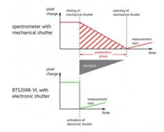
*Electronic Shutter reduces the measurement time*
