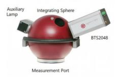
The BTS2048-UV can directly plugged on a integrating sphere (picture shows the constructional identical BTS2048-VL) regards to the communication speed the ethernet port is superior to the USB2.0 interface. Furthermore, the data preparation occurs in the BTS2048-UV-S to optimize the datatransfer speed. For this purpose, an independent, high-performance microprocessor is incorporated.
