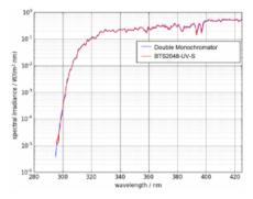
Comparison of a solar measurement of the BTS2048-UV-S and a standard double monochromator. The BTS2048-UV-S achieves about the same quality in a measurement time of a few s compared to about 1.5 min of the double monochromator.
