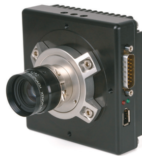
Figure 3 pco.1400 - scientific CCD camera with 1392 x 1040 pixel resolution
