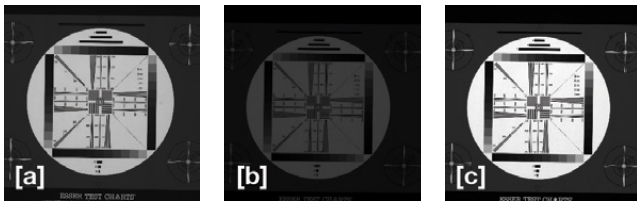
Figure 13: Images of the same test chart with the same resolution, same object distance, and same fill factor but different pixel size, and different lens settings (all images have the same scaling for display):
